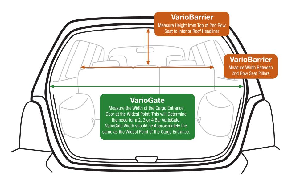
Please note that a Combination of a VarioGate + VarioBarrier is Recommended for the Best Crash Safety
