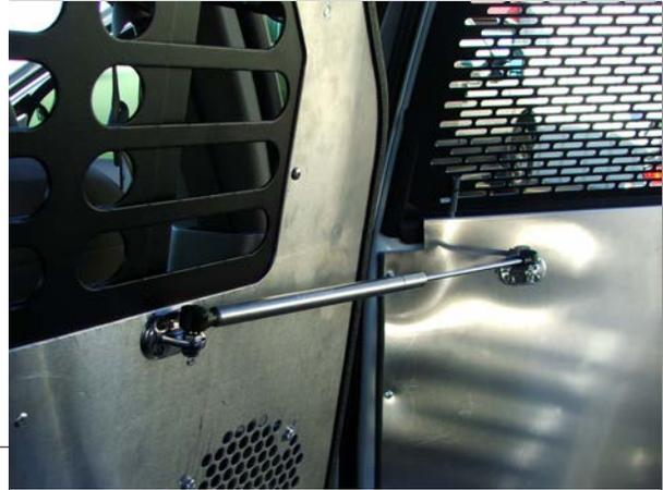
*Drawing 8.11.1: Example Push Rod Mounting Location*
