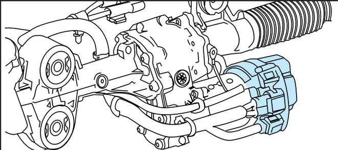
The Electric Power Steering System consists of a Rack-and-Pinion steering gear assisted by an electronically controlled power steering motor and drive assembly. The steering gear is mechanically connected to the steering wheel system.
