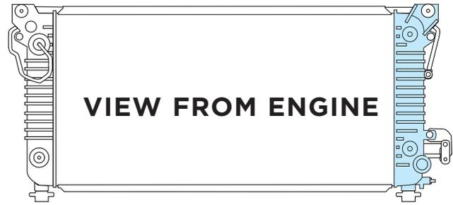
Engine Oil and Transmission Oil are cooled by passing the fluids through separate coolers located in the engine radiator assembly end tank and the air conditioning condenser. Engine oil is pumped by the engine oil pump from the right side of the engine block through piping to an oil-to-coolant heat exchanger located within the right side end-tank of the coolant radiator and returned to the engine. See also TRANSMISSION OIL COOLER.
