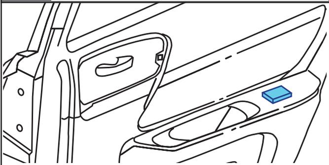
Rear door window switches are inoperable. Rear door power regulators are operable only from driver position switches.
