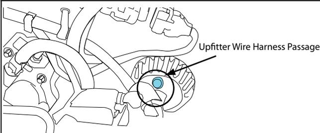
Provides pass through for small number of wires and is located at the lower left side of the front of dash. Carefully remove or puncture only the nipple portion for passage of wire and silicone seal around the wire after installation. Note that a vehicle harness connector is located at the interior side of the grommet and may interfere with passage of wire.
