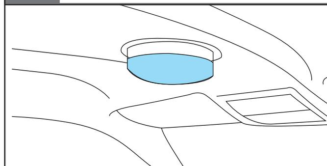
Auxiliary dome lamp is located on the headliner to the rear of the overhead console and is switched at the rear lamp base. Lamp is wired separately standard dome lamps with red and white LED bulbs.
