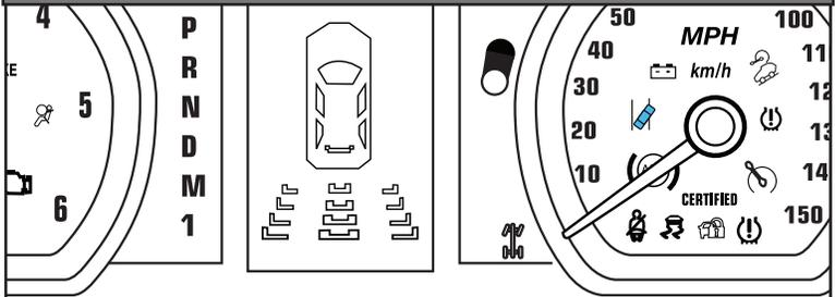
The parking assist displays proximity distance bars to nearby objects. When an object is first detected in the rear, one beep will be heard from the speakers. A continuous beep will sound once object becomes very close.
