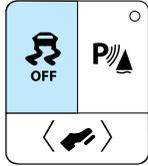
The StabiliTrak Stability Control System control button is located to the left of the steering column on the instrument panel. Button shown is with the optional power adjustable pedals. See also Ride Control Systems in your Owner's Manual for an operation description of the stability control system and related Driver Information Center messages. (See StabiliTrak page for description)
