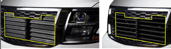
Aero shutters are designed to close when operating conditions permit. The shutters are located on the front of the A/C condenser under hood to divert airflow around the front of the truck reducing wind drag and improves fuel economy. When the cooling system requires more air flow the shutters automatically reopen, ensuring proper air flow through the radiator.
