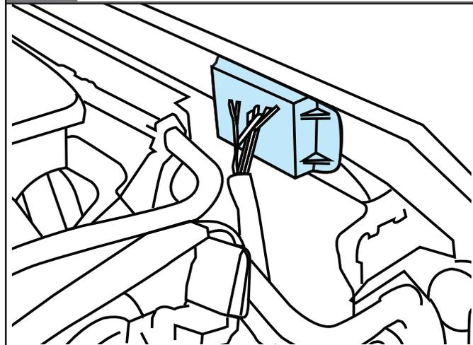
Option 6J7 provides a headlamps high beam flashing module, rear lamps flashing via the Body Control Module (BCM) and a control wire for customer-furnished switching to turn the module on and off. The flasher control wire is part of the blunt-cut upfitter harness coiled under the instrument panel in the front passenger side foot well. The flashing module is located on the rear edge of the right hand upper radiator support.
