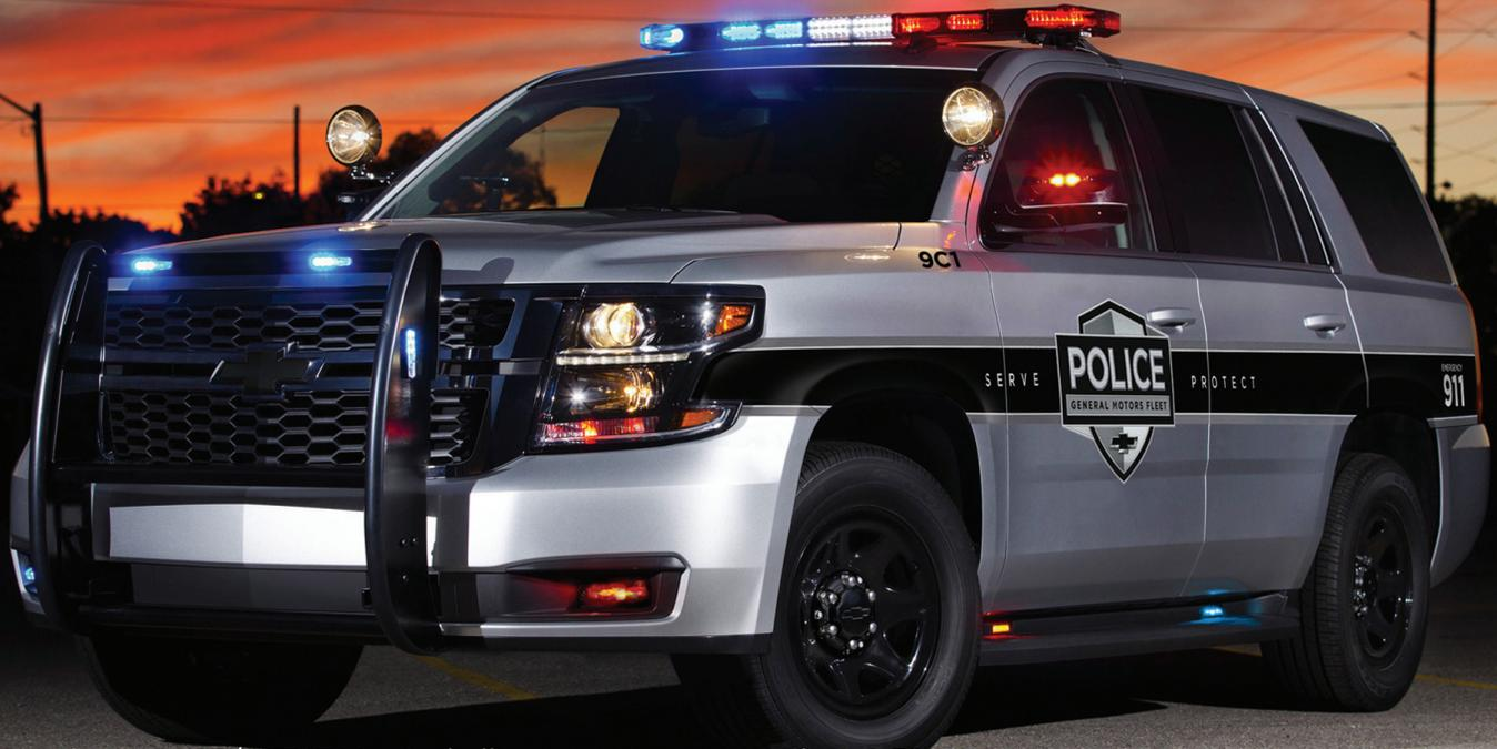
Goodyear P265/60R17 V-rated all season tire mounted on 8.5" black steel wheel with bolted on center cap and matching spare wheel.
