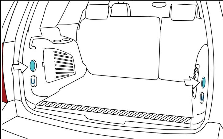
Studs are located on the left and right of the liftgate opening above the tie-down rings
