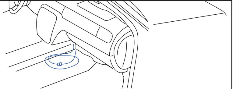
Approximately 60 inches (1.5 m) of auxiliary speaker wiring is routed from the front door and windshield pillar speakers and coiled under the instrument panel. The wiring permits connection of the front speaker pairs to customer-installed communication equipment. Vehicle radio front speaker outputs are re-routed to the rear speakers to maintain the required open door/key-ignition and other audible warnings.
