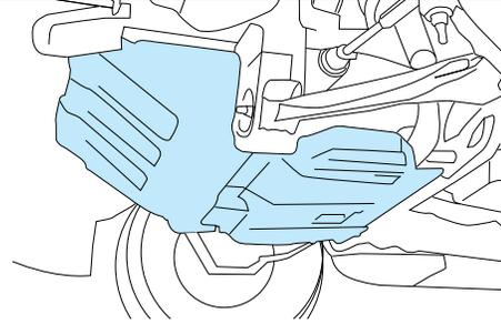
Two piece aluminum front underbody shield starting behind the front bumper and running to the 2nd cross-member protecting front underbody and oil pan.
