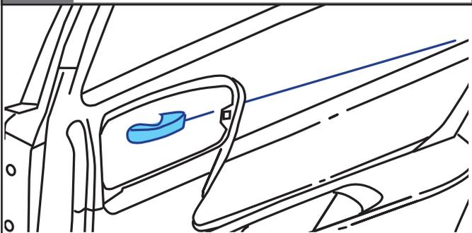
Rear door locking rods are disabled. Rear door locks are inoperable at rear doors, but operate from driver position. Inside rear door handles are disconnected. Rear doors can only be opened from the outside.
