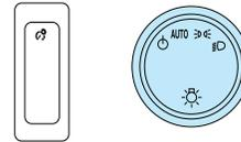
The headlamp control on the driver's side of the instrument panel operates the exterior lamps. If your Tahoe does not have option 9G8, DELETE DAYTIME RUNNING LAMPS and AUTOMATIC HEADLAMPS, the Daytime Running Lamps and Automatic Headlamps can be turned OFF for one ignition cycle by rotating the headlamp control knob momentarily counterclockwise. See also Section 3 of your Tahoe Owner's Manual.
