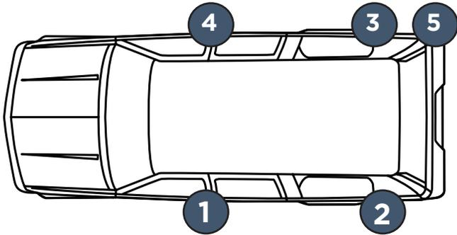
Police Package is equipped with additional grounding in the following locations:
